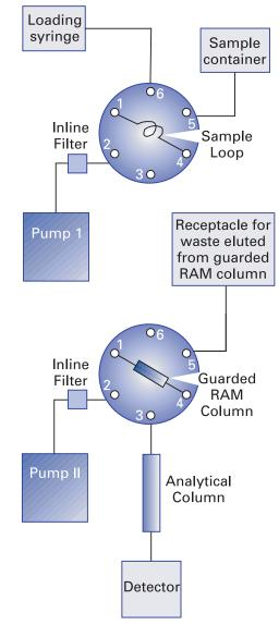
Figure 4. Column switching system.
