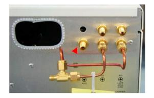
Air tubing from the solenoid is connected to the AIR (luft)
